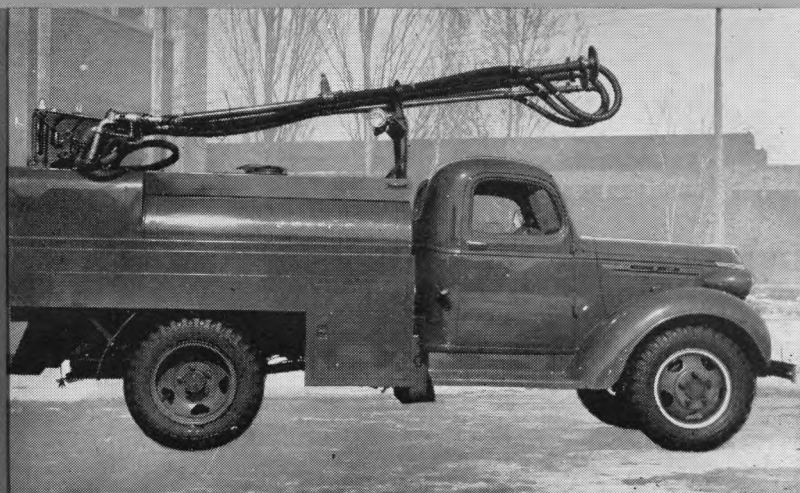
AIRPLANE GASSING TRUCK —A tank body capable of carrying hundreds of gallons of gasoline mounted on conventional chassis used for re-fueling planes at army airports. Special hose racks make it possible to reach gas tanks in big bombers.
